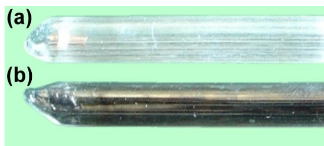
Figure 1. Quartz ampules used for the FMR studies: (a) initial ampule loaded with the sample (a piece of nichrome wire) and organic substrate (1,2-dichloroethane); (b) ampule after the RAPET experiment.
