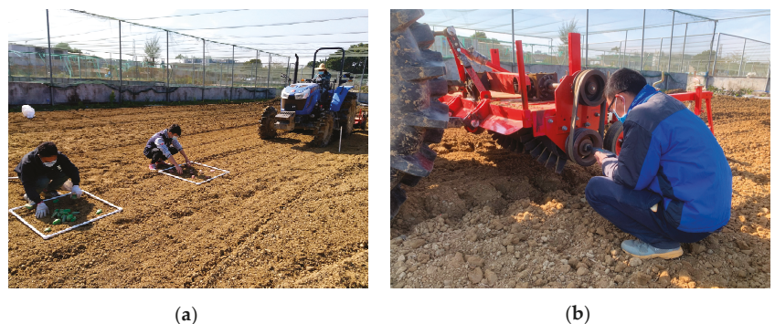
Figure 9. Preparation for the field test: (a) distribution of stone and (b) calibration of operation parameters.
