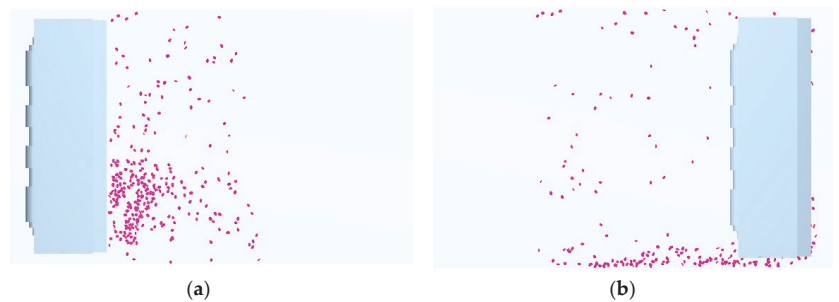
Figure 7. Simulation experiment effect of the device: (a) primary distribution of stones and (b) stone distribution after processing.
