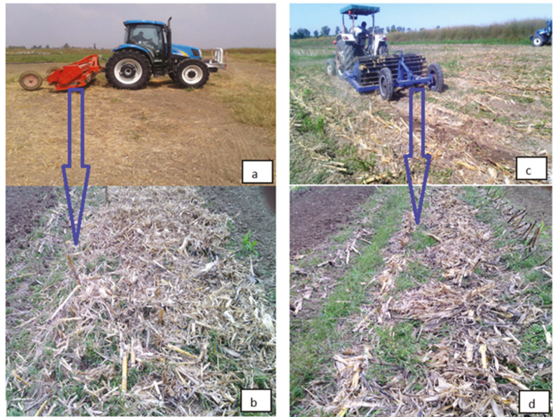
Figure 3. Recorded in experiments: (a) traditional stubble shredder; (b) efficiency of traditional stubble shredder; (c) prototype stubble cutter; (d) images of the effect of the prototype stubble cutter.
