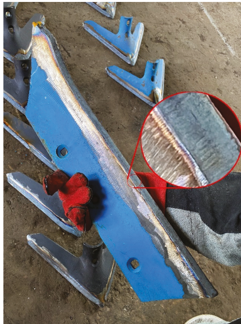
Figure 5. The appearance of the plasma-hardened ploughshare.
