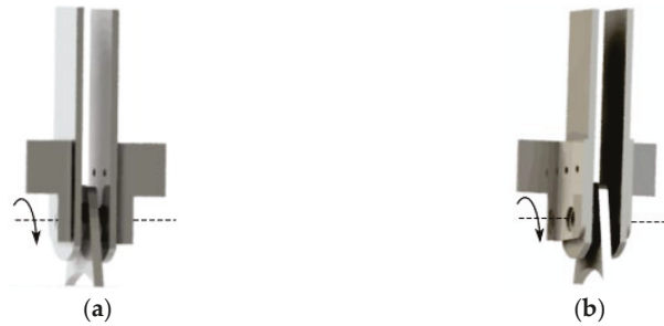
Figure 13. Installation form of wind blades. (a) Forward installation; (b) reverse installation.
