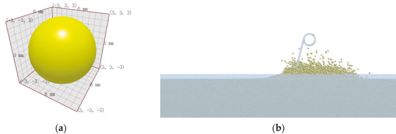
Figure 14. A particle and geometric simulation model. (a) Particle model of the soil; (b) simulation model of the EDEM.
