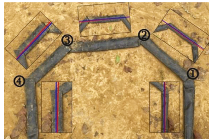
Figure 11. The configuration of the drip tape in the turning area and its detection result (red line). The blue line represented the vertical line in the center of the image. The numbers “①”, “②”, “③”, and “④” represented the corner points, which can divide the drip tape into five line segments.
