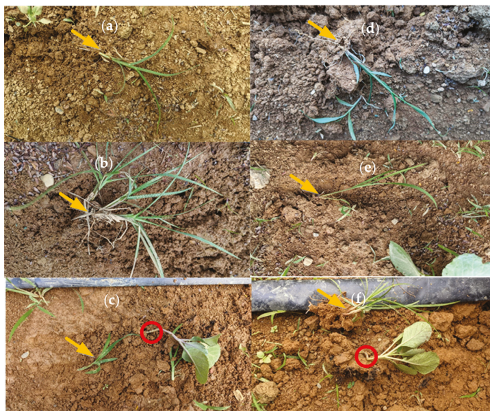
Figure 11. Snapshot of the soil on the field after weeding by the weeding machine. (a) weeds are completely removed by weeder #2, partially removed (b) and damaged crops (c); (d) weeds are completely removed by weeding tool #1, partially removed (e) and damaged crop (f). The red circle and orange arrow indicates the position of the crop roots and the root of the weed, respectively.
