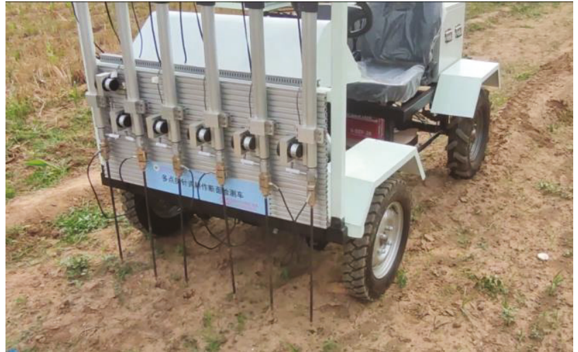
Figure 10. Image of multi-point probe-type tillage section inspection vehicle used in the field test.
