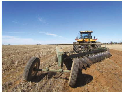
Figure 6. One-way disc plough used in the field tests.
