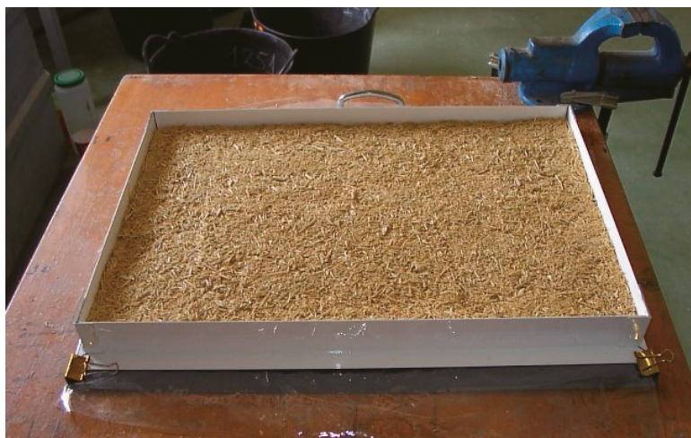
Figure 3. Mat formed manually to manufacture the particleboards.
