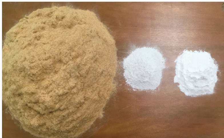
Figure 2. Giant reed (left), gypsum (center), and starch (right) particles used for manufacturing the experimental board type 20:10.
