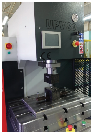
Figure 3. View of forming tool installed in UPV80 hydraulic press.
