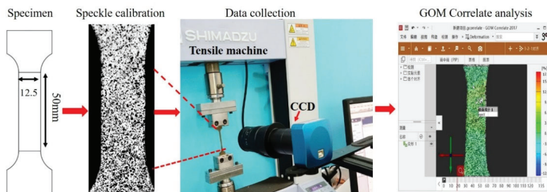
Figure 2. Analysis of the foil deformation process with the DIC technology.
