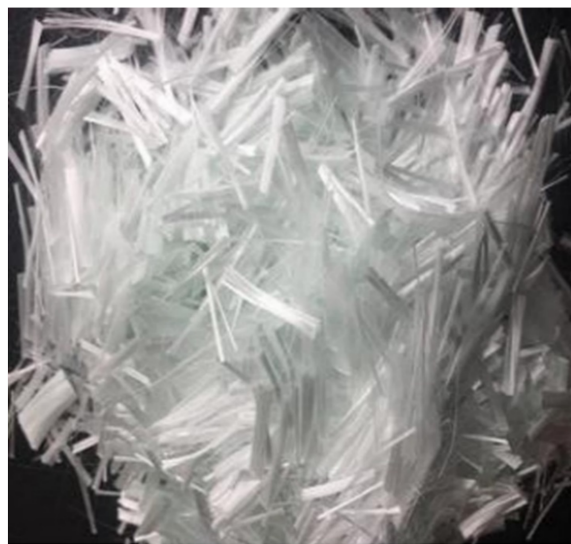
Figure 17. AR glass fibers. Reprinted with permission from Ref. [180]. Copyright 2021, with permission from Elsevier.
