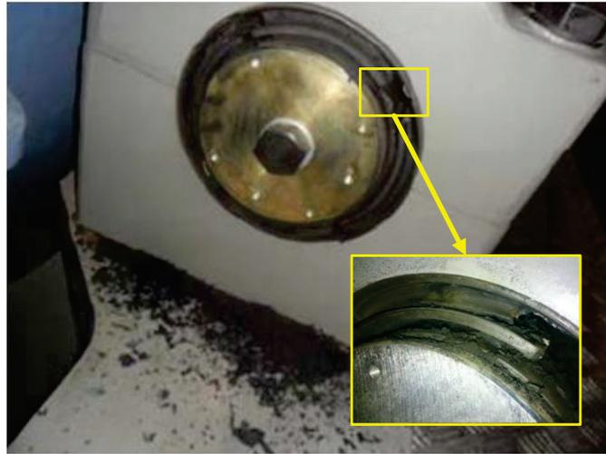
Figure 10. Main bearing offset failure.
