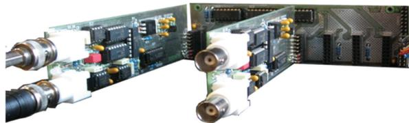
Figure 3. Hot-wire anemometer with automatically adjusted dynamic properties.
