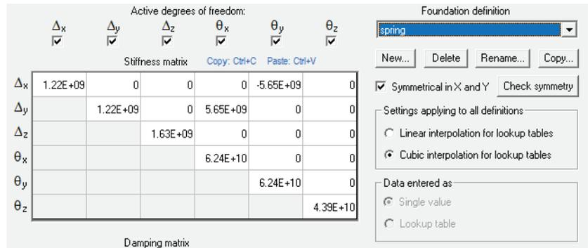
Figure 7. Bladed input for stiffness of foundation spring.
