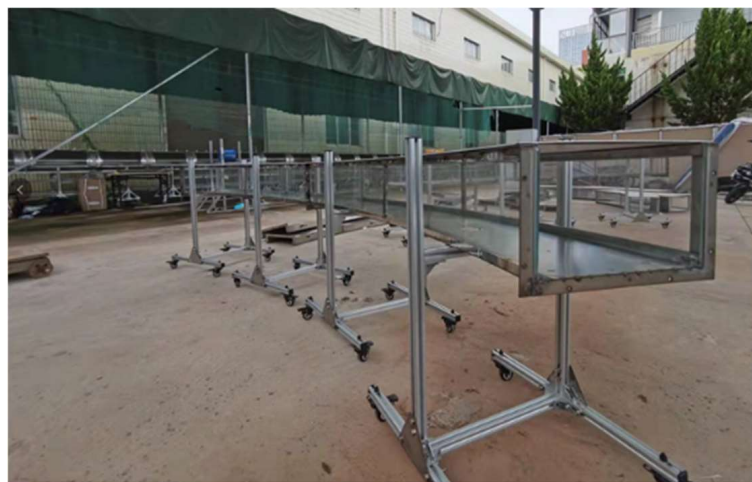
Figure 1. Apparatus of small-scale curved tunnel.
