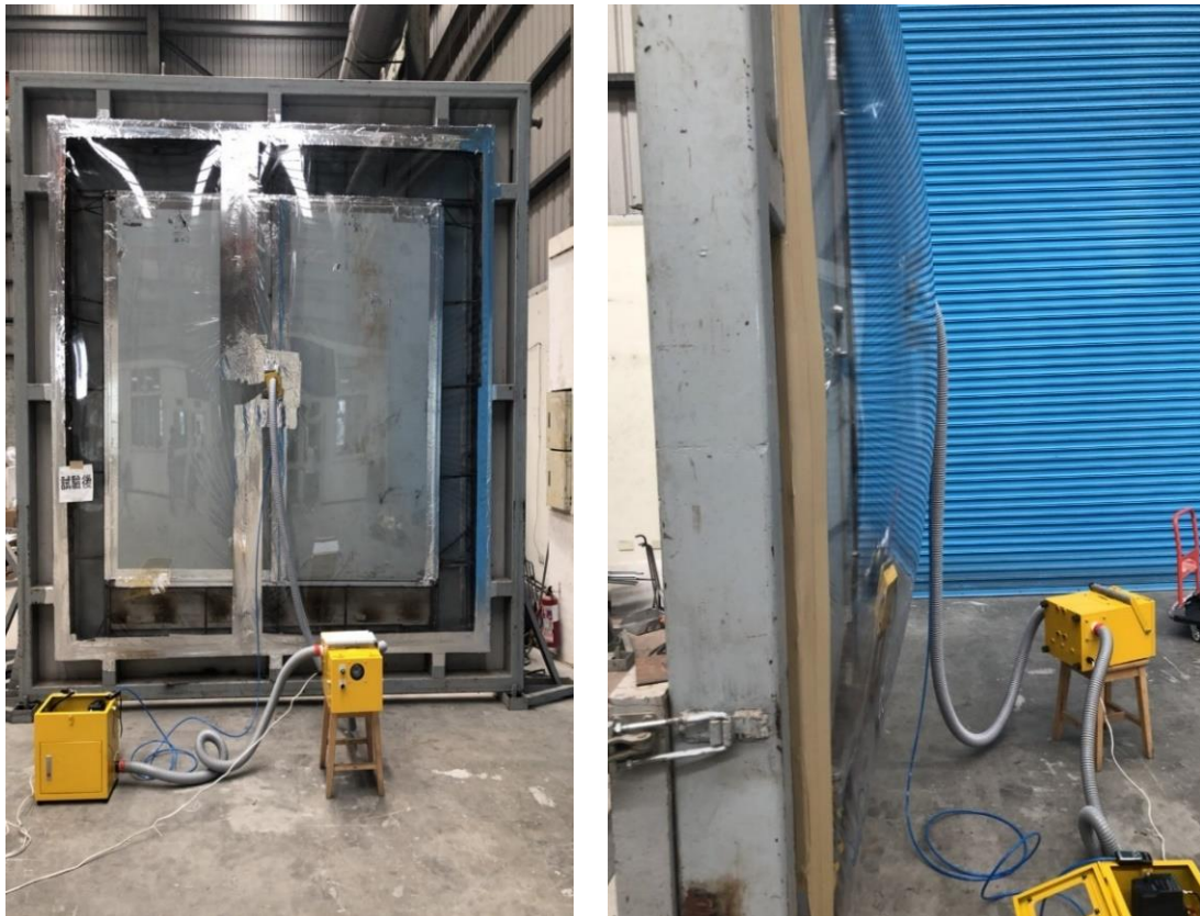
Figure 4. Smoke control field test method verification.
