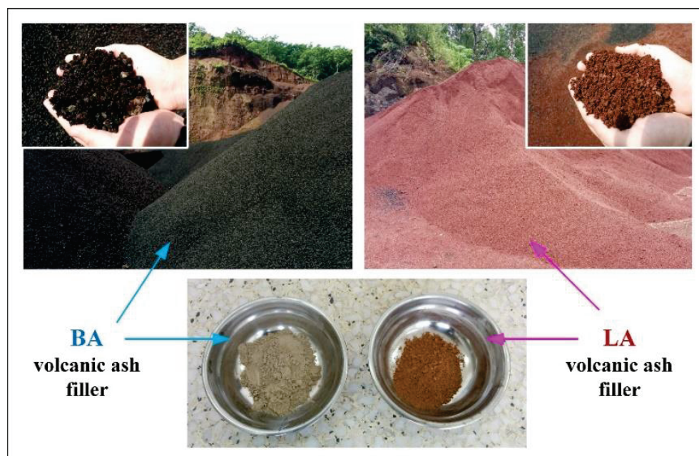
Figure 1. The volcanic ash fine filler of Bahaozha (BA) and Lazihe (LA).
