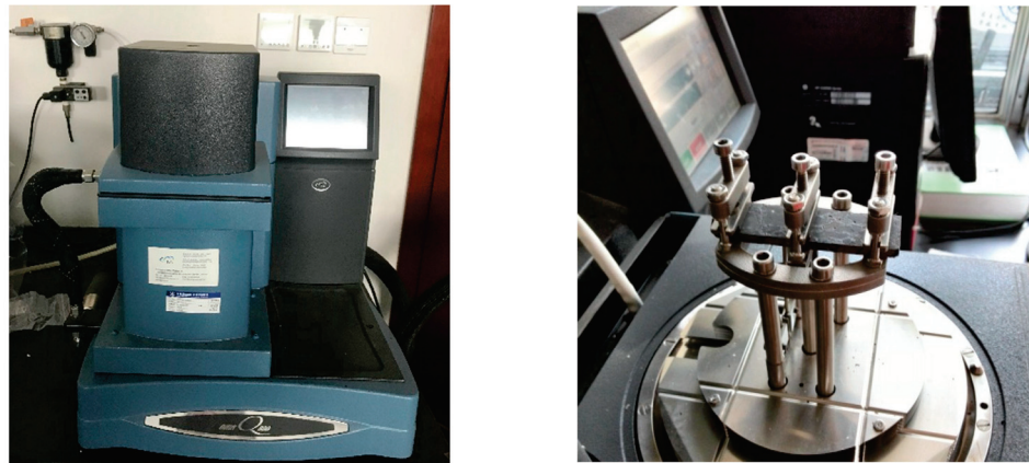
Figure 2. DMA instrument and dual cantilever clamp.
