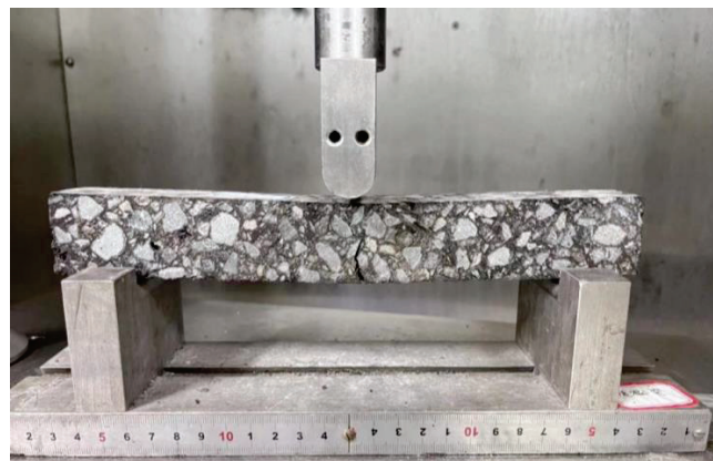
Figure 5. Low-temperature bending beam test.
