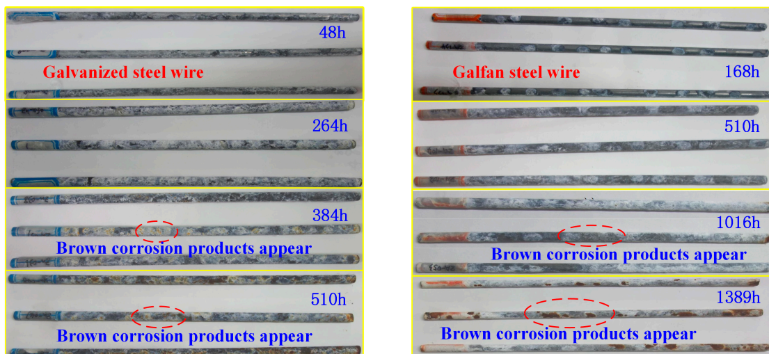
Figure 3. Corrosion morphology in the different stages of corrosion.
