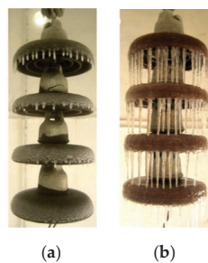
Figure 22. Results of 4-h icing with and without a coating of insulators. (a) With coating. (b) Without coating [49].
