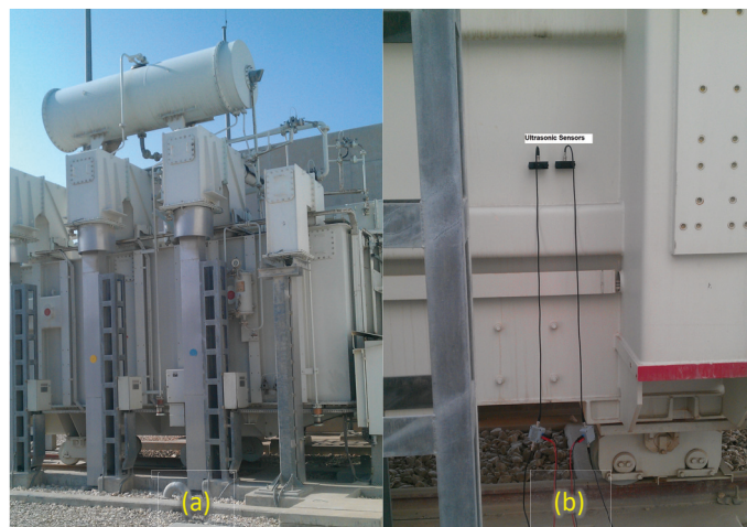
Figure 9. (a) A photo of a power transformer, (b) acoustic sensors installed on the tank of a transformer.
