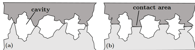
Figure 7. Illustration of surface asperities leading to cavities and contact spots at solid–solid interfaces at (a) no-load, (b) increased contact area and reduced cavity size under load. Reproduced from [12], Macedonian Journal of Chemistry and Chemical Engineering: 2018.
