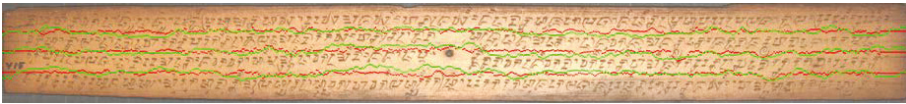
Figure 25. Text line segmentation of Sundanese manuscript with the Seam Carving method (green) and Adaptive Path Finding (red).
