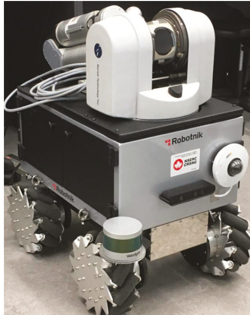
Figure 5. The omni-directional mobile robot used to validate the monocular VO algorithm with the proposed pipeline.
