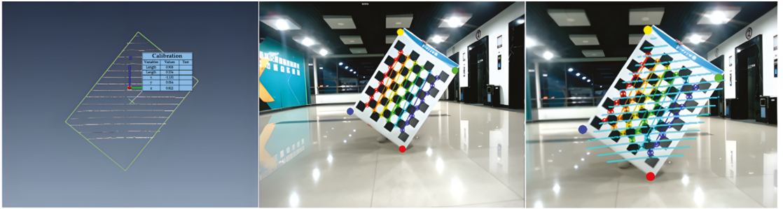
Figure 6. The coordinate system calibration of the multi-source sensors.
