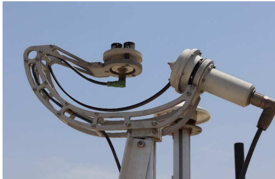
Figure 3. CSPC Twin-RSI installed at UET Peshawar.
