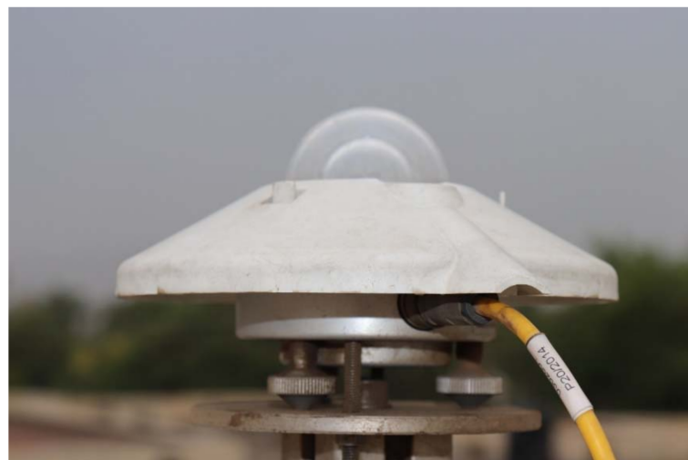
Figure 2. Kipp & Zonen CMP10 pyranometer installed at UET Peshawar.
