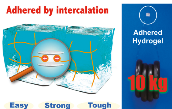
Figure 4. Schematic representation of high concentration cationic gels adhered using 1.6 mg of Micromica supporting a tensile load of 10 kg. Reprinted from [81] with permission from the American Chemical Society (2016).
