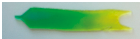
Figure 1. Demonstration of colormetric gradient in a polyethylene glycol hydrogel. Adapted with the permission from [73]. Copyright 2015 Elsevier.
