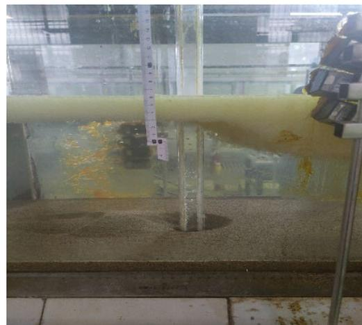
**Figure 4.** Local scour hole around a pier.
