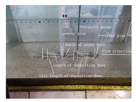
Figure 2. Measurement using a point gauge.
