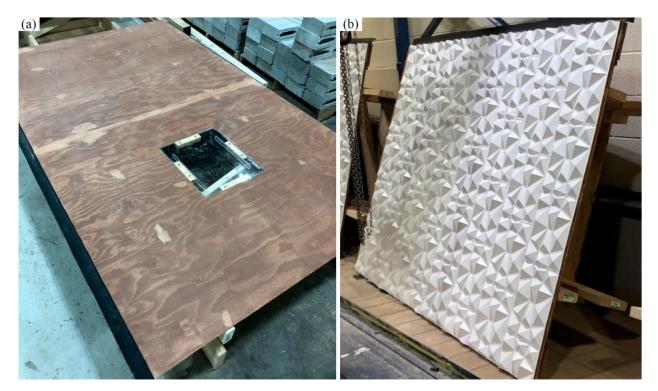
Figure 3. Bottom surface of the ice cover: (a) smooth condition, and (b) rough condition.
