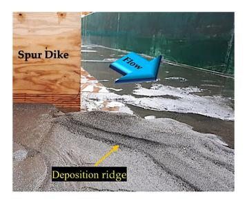
Figure 6. Deposition ridge in the downstream side of the spur dike.
