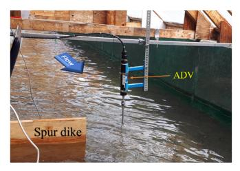
Figure 3. 3D Velocity data collection using the 10-MHz SonTek ADV.
