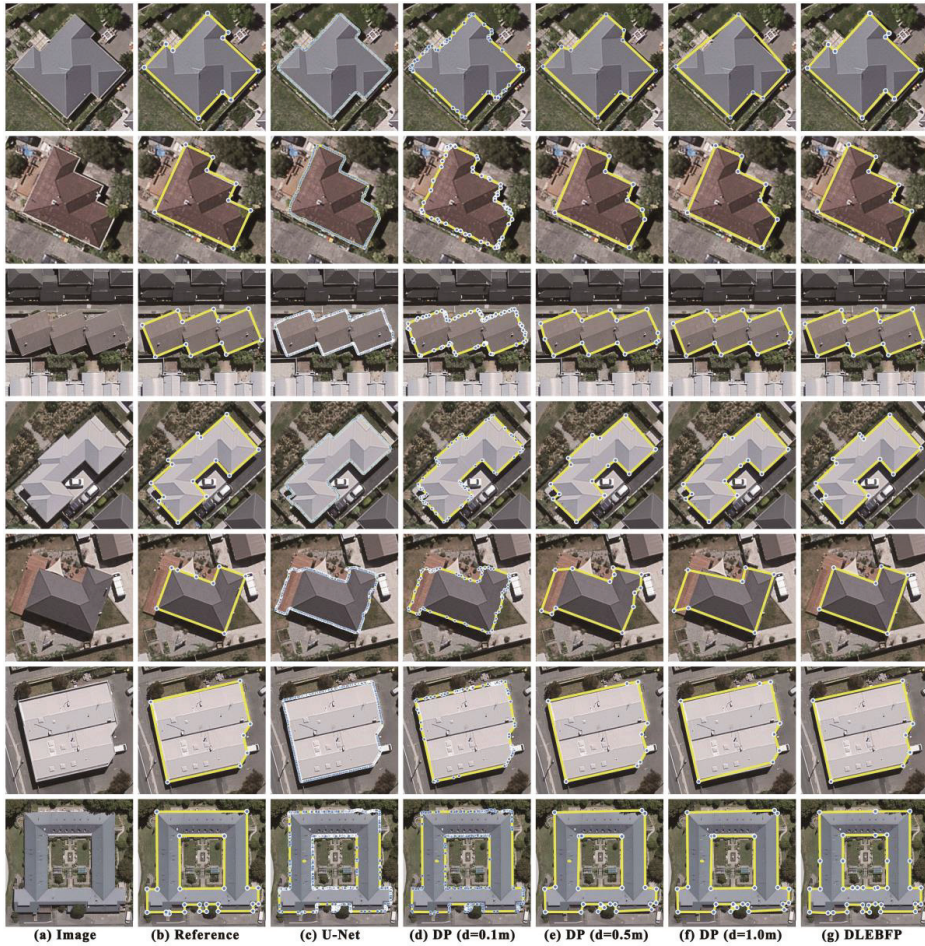
Figure 5. Examples of the true-color-composite images and extracted building footprint polygons using different methods on the WHU dataset are shown for (a) the true-color composite images, (b) the ground reference images, (c) the polygons derived from U-Net, (d–f) the polygons derived from U-Net and simplified by Douglas Peucker algorithms with 0.1, 0.5 and 1.0 m threshold, (g) the polygons derived from DLEBFP. The building footprint boundaries and vertices are marked by yellow lines and blue dots, respectively.
