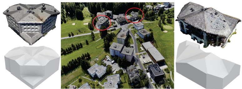
Figure 11. Reconstruction from aerial point clouds. In these point clouds, the vertical walls can be extracted from the point clouds and directly used in reconstruction, and thus the vertical plane inference step was skipped. The dataset is obtained from Can et al. [56].
