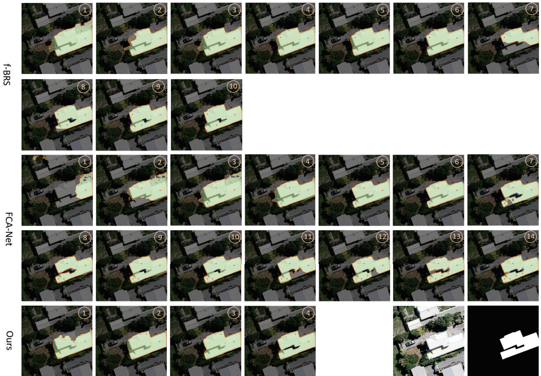
Figure 13. Visualized comparison of the segmentation process of f-BRS, FCA-Net and our algorithm on a test case of AIRS dataset. Red for positive clicks and blue for negative clicks.
