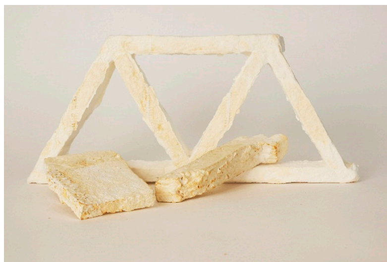
Figure 11. Truss structure made from cellulose pulp.
