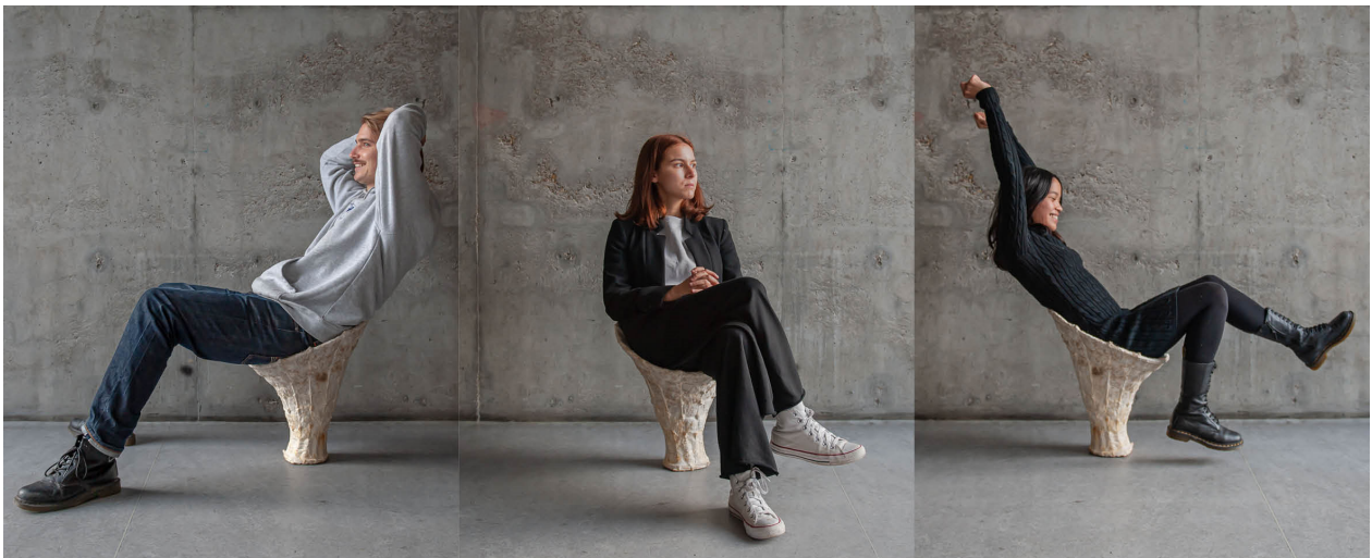
Figure 15. Seating tests (44 to 90 kilos).
