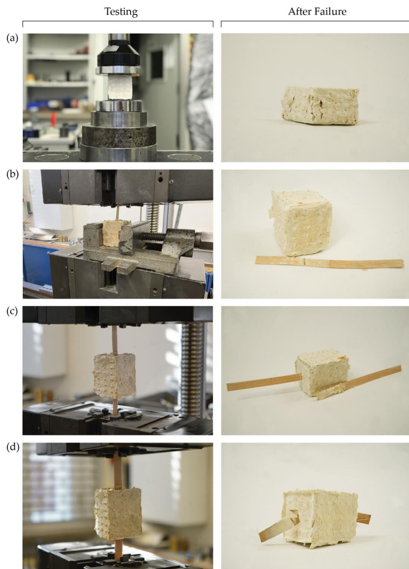
Figure 7. Samples during testing and after failure: (a) Compressive strength test; (b) One-side veneer pull-out test; (c) Two-side unwelded veneer pull-out test; (d) Two-side welded veneer tensile test.
