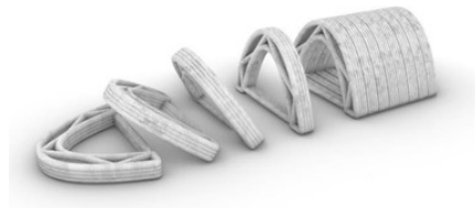
Figure 11. The concept design of the extruded vault (Image credit: Authors).
