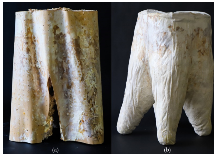
Figure 1. Mycelium-based prototypes: (a) using a timber veneer mold, and (b) using cotton fabric mold, by F. Milano, K. Antorveza, L. Kiesewetter, G. Lochnicki, Materials Matter Lab IV, 2020.
