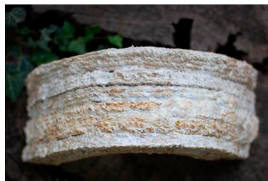
Figure 15. The Bio-welded Arches (Image credit: Authors).
