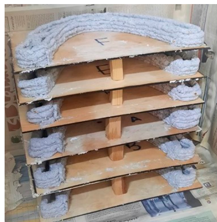
Figure 13. The printed arches growing in the chamber (Image credit: Authors).
