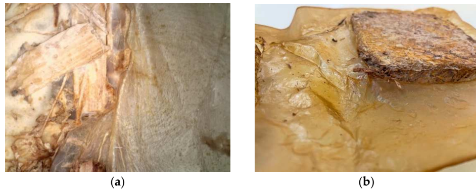
Figure 5. (a) Dried BC around oven-dried mycelium tile under the Dino-Lite digital microscope. (b) Large BC sheet dried around mycelium tile (image credit: authors).
