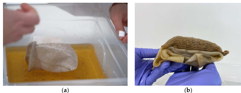
Figure 3. (a) The knitted pocket being placed inside the kombucha culture on top of the acrylic scaffold with the top half being lifted. (b) Pocket filled with pre-inoculated mycelium substrate and BC folded in 9 layers underneath (image credit: authors).
