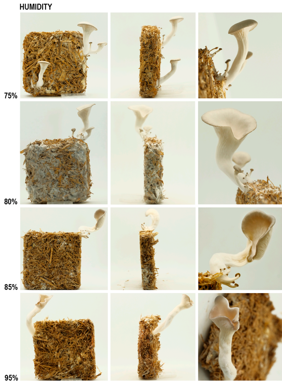
Figure 5. The results of the humidity experiment, front (column 1), side (column 2) and detailed (column 3).
