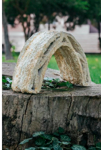
Figure 14. The extruded vault made of MBC material bound by bio-welding (Image credit: Authors).
