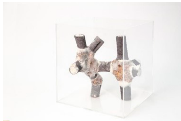
Figure 4. The Bar-node Structure Fabricated with Mycera (Image credit: Julian Jauk, Hana Vasatko, Lukas Gosch).
