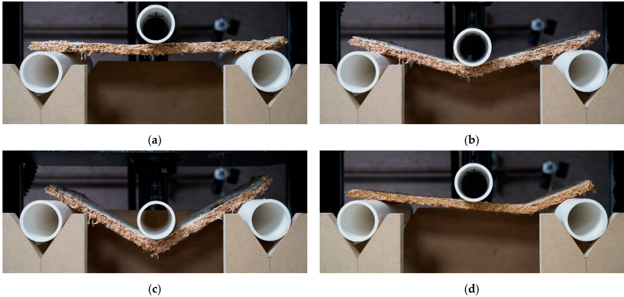
Figure 7. This figure shows the deformation of a PO_LNCB specimen throughout the bending test: (a) beginning of the test; (b) after 6 min and 25 s; (c) after 13 min (just before the end of the test). (d) shows the asymmetric deformation of a different specimen from the PO_LCD sample after 3 min.
