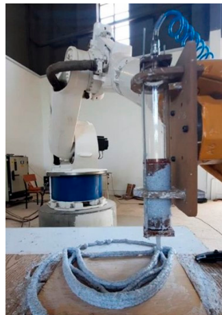
Figure 12. The printing session of one of the arches (Image credit: Authors).
