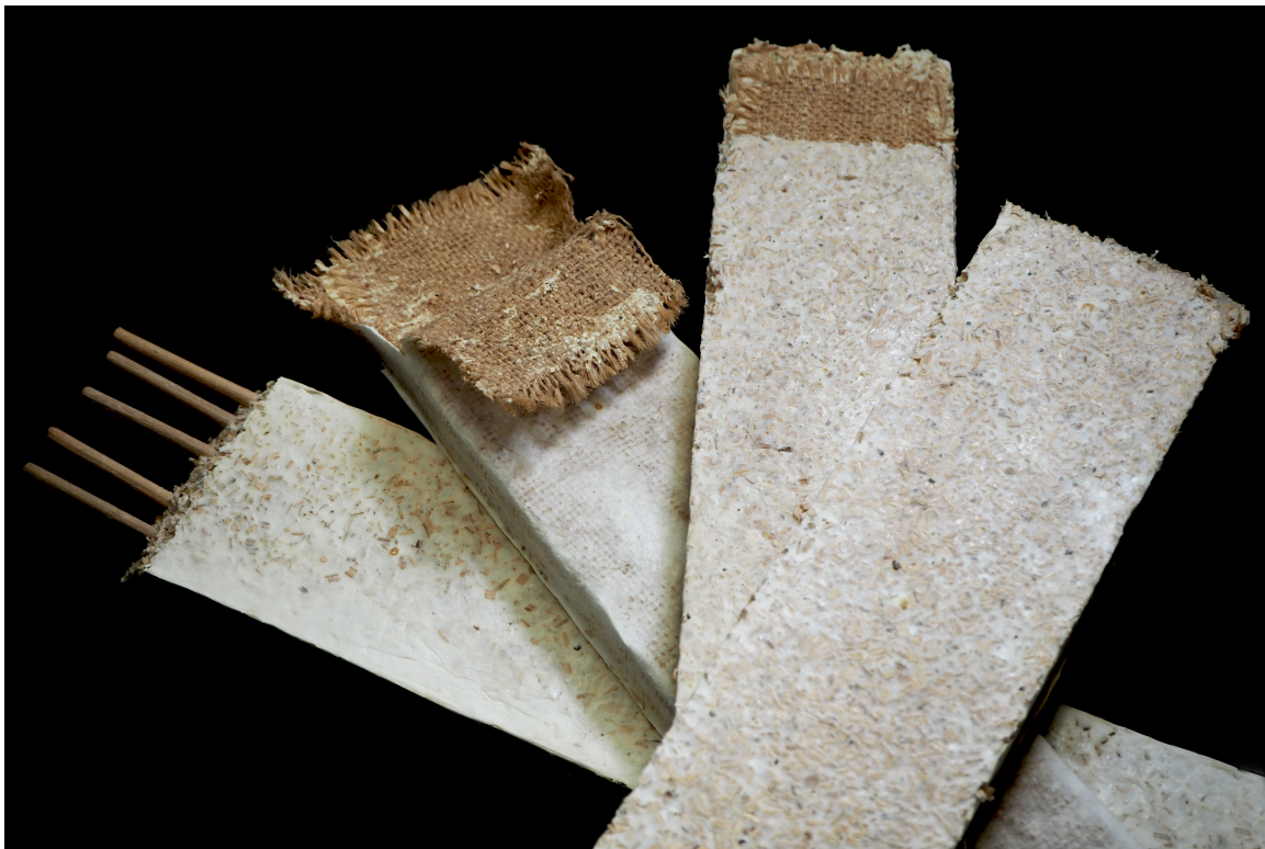
Figure 2. Fibre placement strategies in tested specimens (left to right): rattan fibres (BM_R), hessian jacketing (BM_H), inner hessian (BM_I), control (BM).
