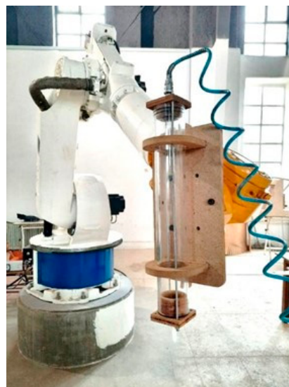
Figure 8. The Fabricated Extruder (Image credit: Authors).
