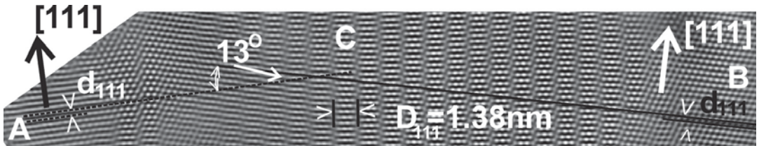
Figure 6. High-resolution TEM micrograph from two partially overlapping [111] type whiskers A and B; the overlapping area is denoted by the letter C. The observed rotational Moiré pattern has a periodicity of D_{111} = 1.38 nm.
