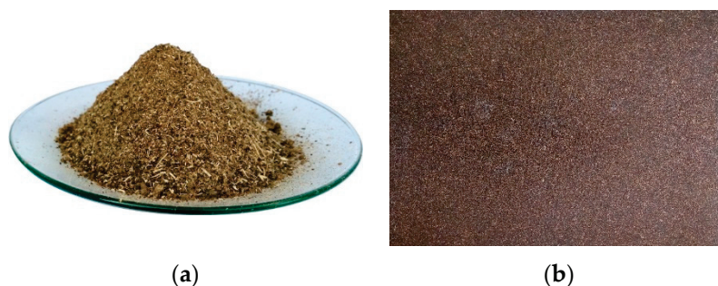
Figure 3. (a) Dry-compounded feedstock and (b) sample board, after hot-pressing at 180 °C for 30 min.
