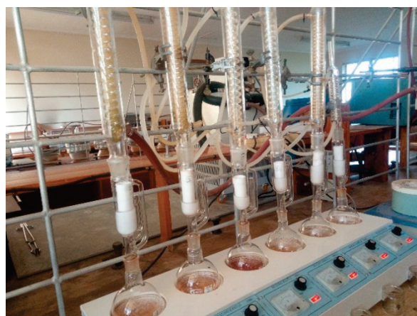
Figure 5. Soxhlet extraction setup for biomass compositional analysis.
