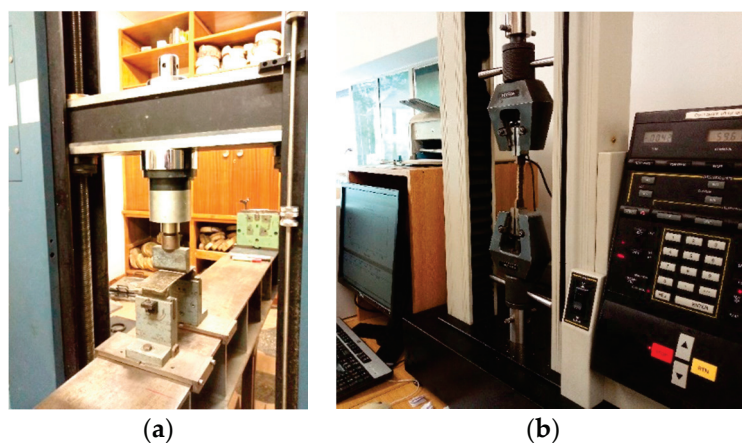
Figure 6. Instron setup for (a) the 3-point bending test, and (b) tensile test.
