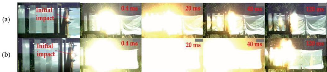
Figure 17. Comparison of high-speed images of RMP hitting MLAT: (a) hitting a 2 mm RHA steel target at a speed of 936 m/s and (b) hitting a 15 mm RHA steel target at a speed of 940 m/s.
