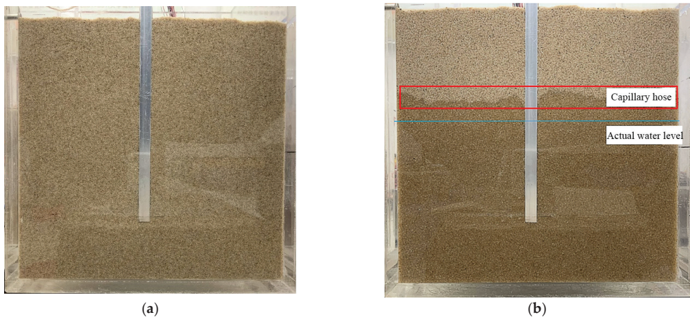
Figure 3. The sand packed in the box. (a) Packed sand. (b) Packed sand with groundwater.
