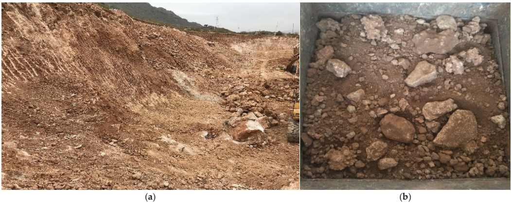
Figure 1. SRM in Zhaizi village, Lijiang City, Yunnan Province, China. (a) Site investigation; (b) SRM sample.
