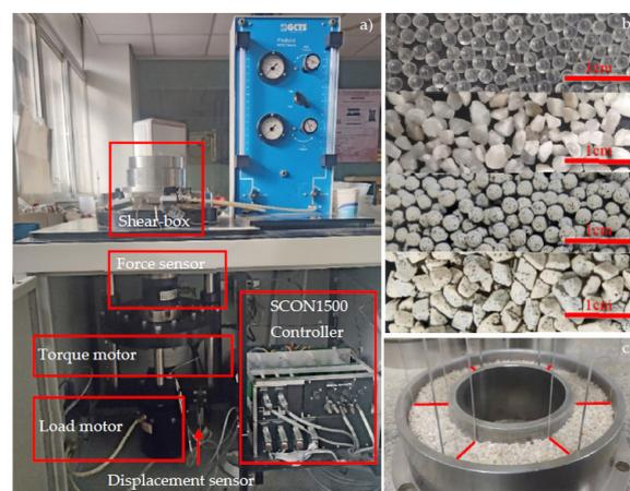
**Figure 1.** The basic condition of the ring-shear test. (a) Structure of GCTS ring-shear apparatus; (b) Initial photos of experimental materials; (c) Partition filling method. This figure was modified from Huang et al. [24].
