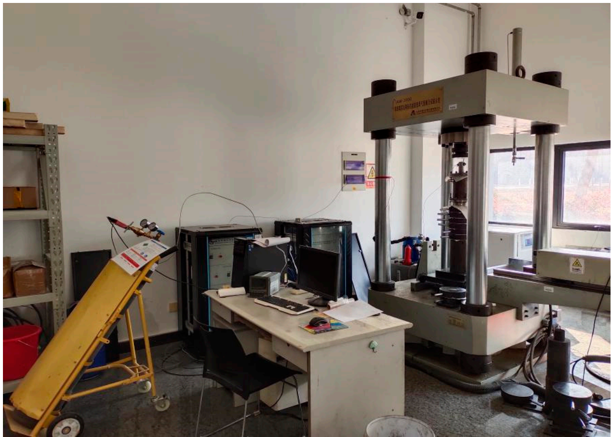
Figure 2. TAWD-2000 coal rock mechanics-seepage triaxial test system.
