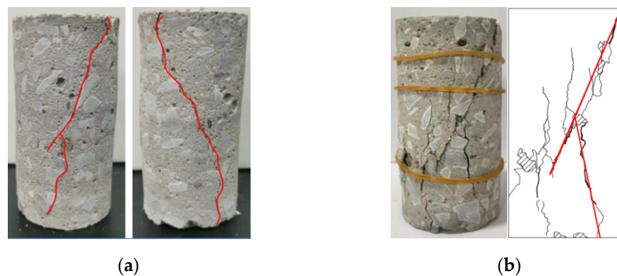
Figure 5. Fracture characteristics of back-filling concrete samples under different loading paths. (a) J-1 sample uniaxial loading path; (b) J-11 sample under cyclic loading path.
