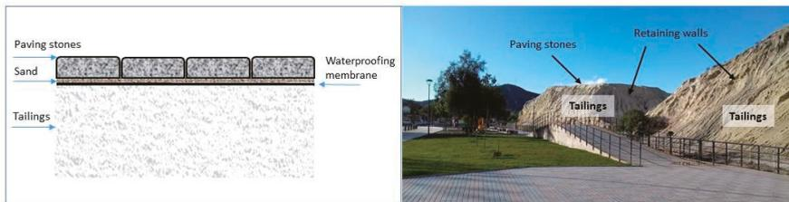
**Figure 1.** Scheme for using paving stones. The figure on the left shows a graphic. The figure on the right shows the proposed tailings surface coverage system at Andacollo commune.
