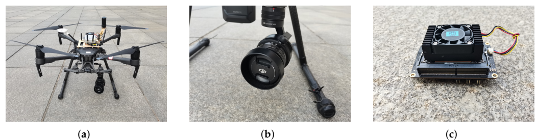
Figure 11. Hardware system for flight experiments. (a) DJI Matrice M210v2 drone; (b) DJI camera; (c) Nvidia Jetson Xavier NX.
