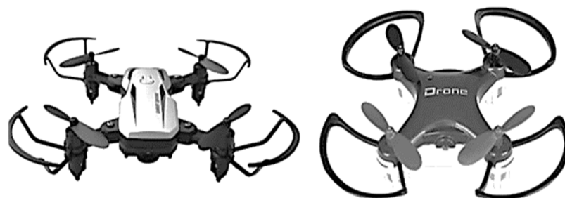
Figure 9. UAVs with closed and safety propellers.
