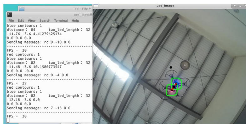
Figure 13. Monitor image processing, red and blue LEDs indicated by the green circle.
