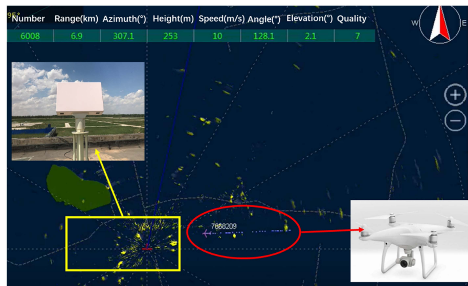
Figure 2. Example of tracking trace of the drone on the radar (i.e., Radar- \gamma ) screenshot.
