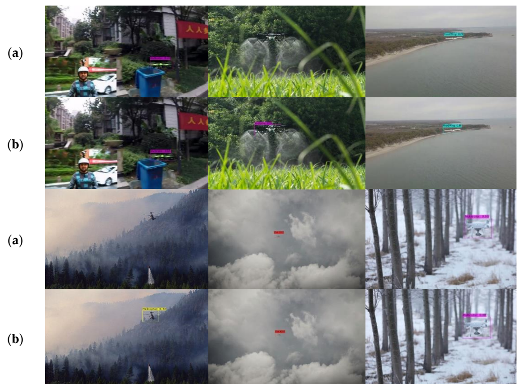
Figure 20. Several samples of drone recognition in different light and weather conditions and against a crowded background. (a) YOLOv4. (b) Modified YOLOv4.
