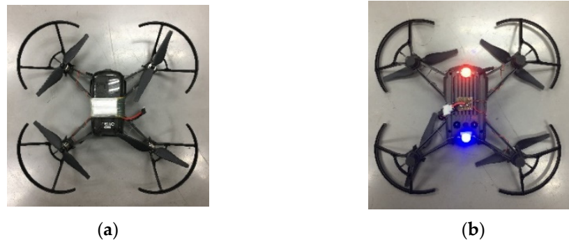
Figure 1. Tello EDU and two LEDs with different colors were installed on the bottom of the drone. (a) Top view; (b) Bottom view.
