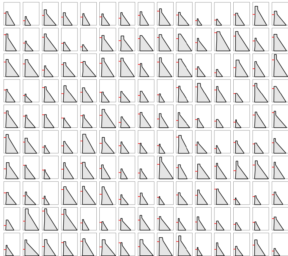
Figure 3. Inventory of all gravity dam shapes generated based on a Matlab code including a random water level in red; the box size is 170 \times 240 m in all cases.
