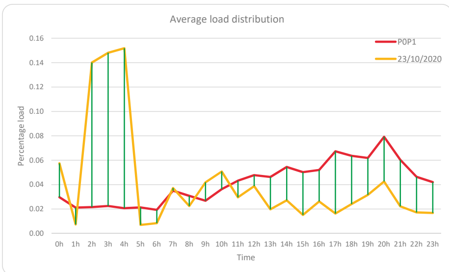
Figure 19. Average load distribution for each hour of the day and the scenario without load shifting or habit adaptation (P0P1 series). The load distribution for day 23 October 2020 has been added as an example to obtain the net load shifting.
