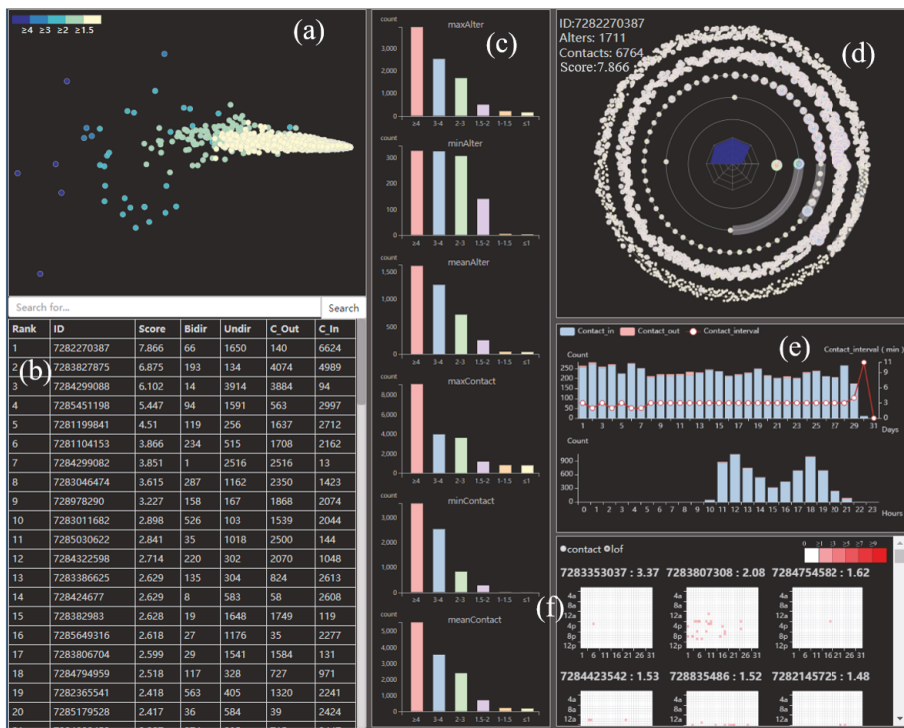
Figure 4. The overview of egoDetect based on the call record data. The user interface consists of six parts: (a) The distribution of users with their features, (b) a list sorted by users’ anomaly scores, (c) statistical information for each segment, (d) the ego network glyph inspired from solar system, (e) the statistical view of ego’s active time and behavior, (f) the detail view about the contact between the ego with each alter.
