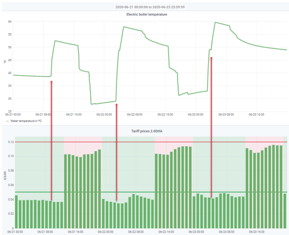
Figure 8. Heating of the water in the electric boiler during the most economical hours. The heating cycle of the boiler is displayed, and the heating hours are marked. Data from 21 June 2020 00:00:00 to 23 June 2020 23:59:59.
