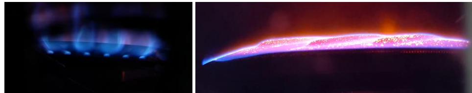
Figure 13. Standard water heater (Left, Steady State) and ULN Water Heater #2 (Right, 30 s After Ignition) operating in situ with 30% H 2 .
