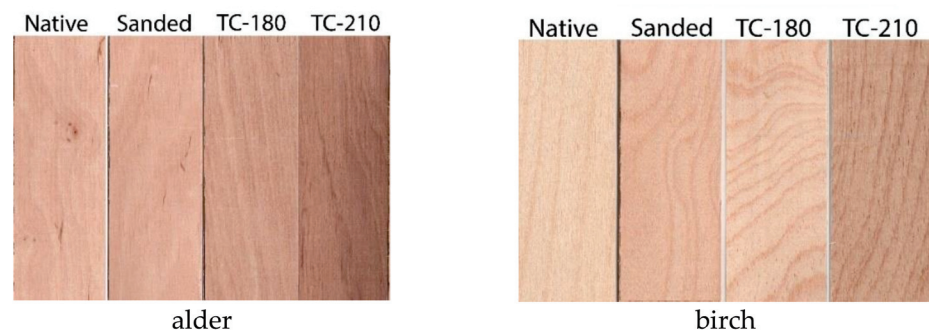
Figure 2. Visual appearance of the surface of alder and birch veneers, native, sanded and thermally compressed at different temperatures.
