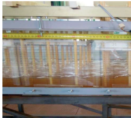
Figure 2. Laboratory flume with arrays of cylinders representing rigid vegetation, University of Calabria.
