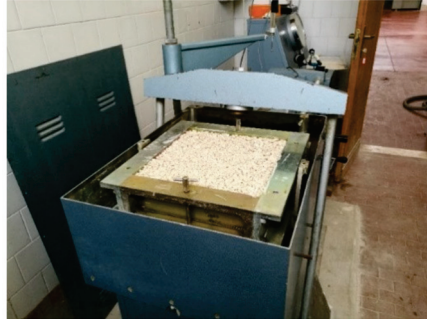
Figure 11. Box used for the cutting tests.
