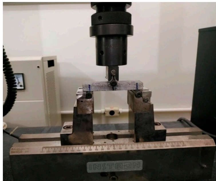
Figure 2. Specimen during the three-point bending test.
