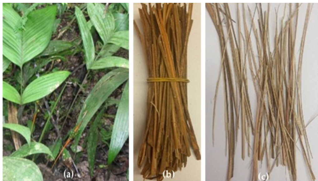
Figure 1. Ubim (a) plant, (b) mechanically divided splints from the stalk, and (c) bunch of final separated and isolated fibers.
