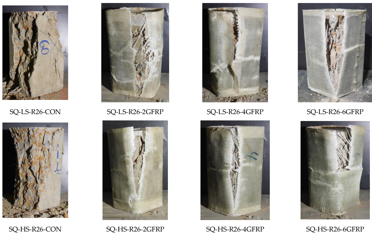
Figure 6. Ultimate failure modes of Group 2 specimens.
