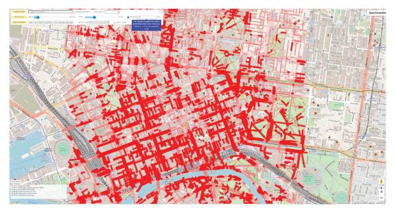
Figure 6. Screen capture of PedestrianCatch displaying topographic analysis of gradients with maximum gradient set to 1:20. (red colour indicates inaccessible road segments).
