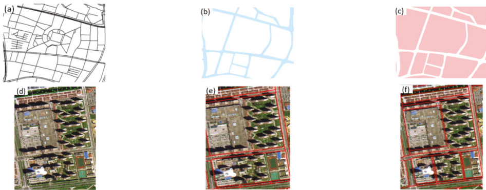
Figure 5. Road network processing and block generation: (a) original OSM road network; (b) road buffers from OSM; (c) segmentation results based on OSM road buffers; (d) raw image; (e) the OSM before editing; and (f) the OSM after editing.
