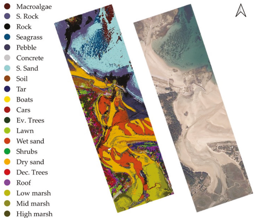
Figure 9. Projected 3D map of the habitats obtained with the predictions of a random forest classifier on green spectral features, infrared intensities, and elevation values; orthoimage of the study area. The orthoimage was captured in 2014, while lidar data are not contemporaneous as they date from 2019. S. = submerged, Ev. = evergreen, Dec. = deciduous.
