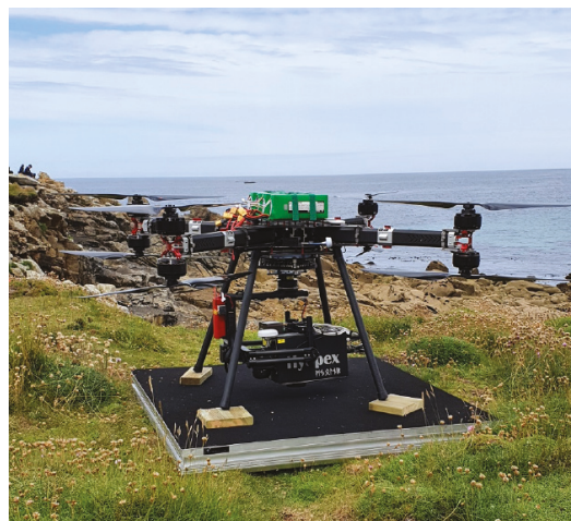
Figure 2. UAV octocopter used for the acquisitions.
