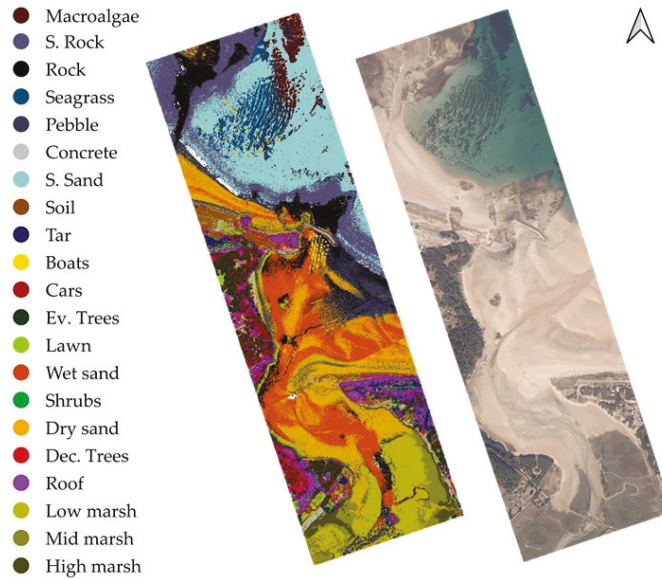
Figure A3. Projected 3D map of the habitats obtained with the predictions of a random forest classifier on green spectral features and elevation values; orthoimage of the study area. The orthoimage was captured in 2014, while lidar data are not contemporaneous as they date from 2019. S. = submerged, Ev. = evergreen, Dec. = deciduous.
