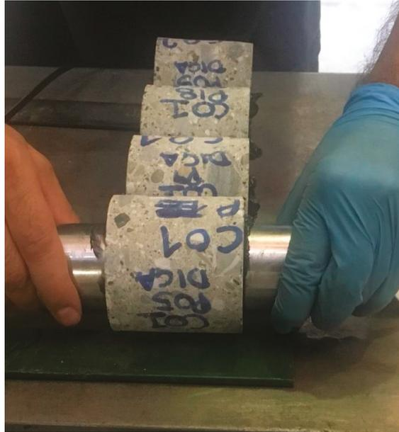
Figure 10. Direct measurement of ultrasonic velocity on single concrete samples.
