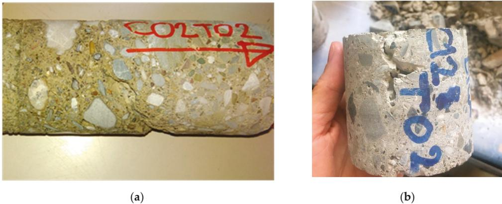
Figure 6. High porosity concrete in extracted samples: (a) Column, (b) Beam.
