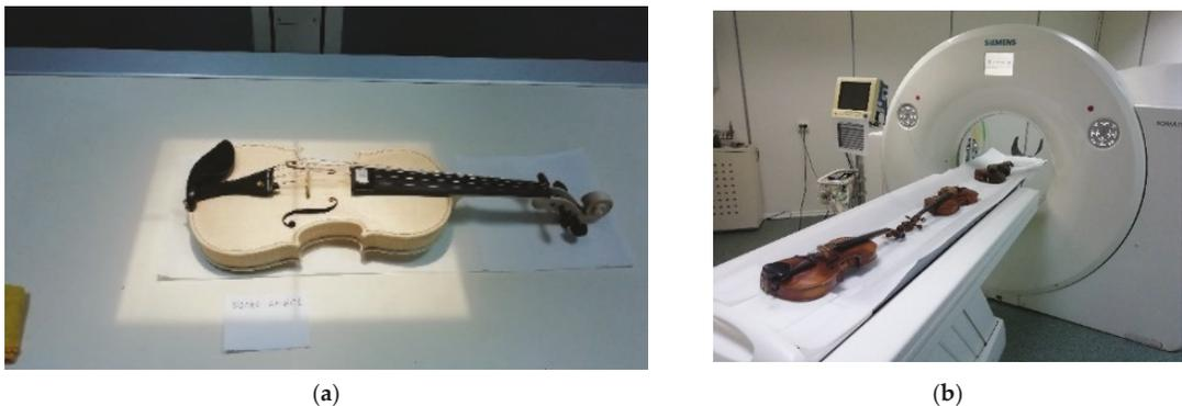
**Figure 5.** Old violins analyzed using non-invasive and non-destructive methods: (a) X-ray of the violin; (b) Computed Tomography analysis of old violins.
