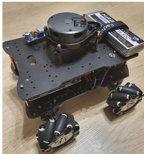
**Figure 3.** Omni-mecanum-wheeled robot.
