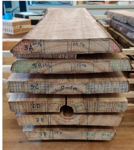
**Figure 3.** Marking of Paulownia sawn wood in the cross-section prior to the preparation of testing specimens.
