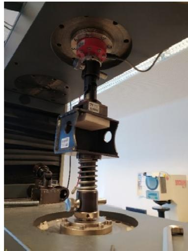
**Figure 2.** Measuring of the screw withdrawal resistance of a Paulownia sample from Spain with universal testing machine Zwick Roell Z 250.
