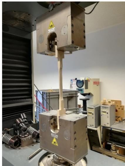
**Figure 1.** Measuring of the tensile strength of a Paulownia sample from Bulgaria with universal testing machine Zwick Roell Z 250 (in the background the device Emco Test Automatic for testing of Brinell hardness).
