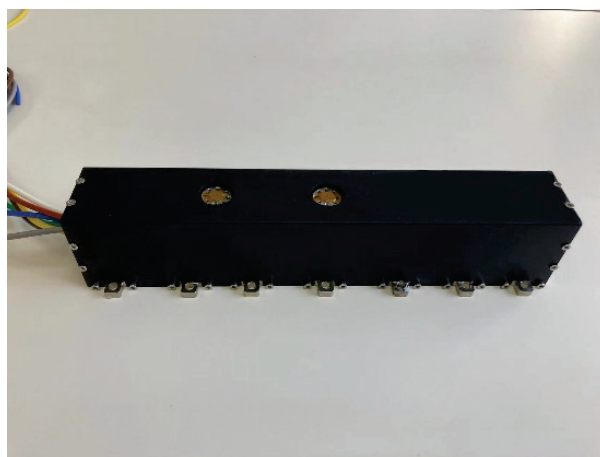
Figure 21. The photo of the packaged G-band TWT.
