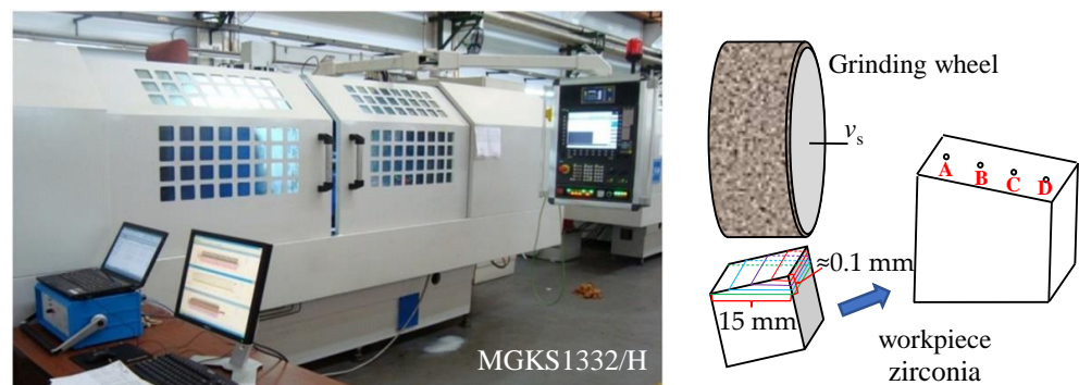
Figure 3. Experimental setup for high-speed grinding.
