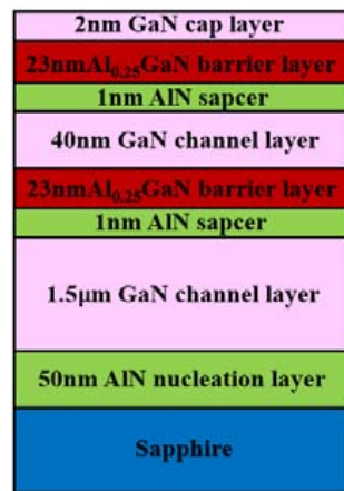
Figure 3. Diagram of the double channel epitaxial layer.
