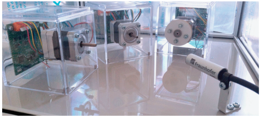
Figure 14. Three electric motor setups for IDMT-ISA-ELECTRIC-ENGINE dataset [14].
