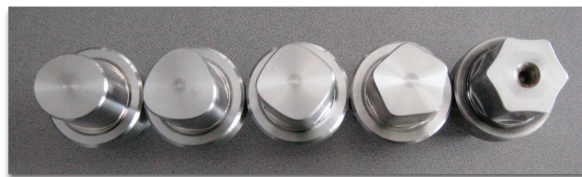
Figure 2. Some H-profiles manufactured by two-spindle process, Iprotec GmbH, © Guido Kochsiek, www.iprotec.de , Zwiesel, Germany [5].
