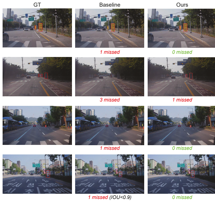
Figure 11. Qualitative results on CSS138 validation set. From left to right, each row shows ground truth (GT), the baseline (naive cut-and-paste), and Ours. For each result on the baseline and ours, we denote the number of missed construction signs.
