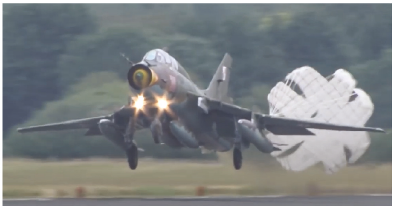
Figure 16. Examples of landings with prematurely opened drogue parachute [29–31].
