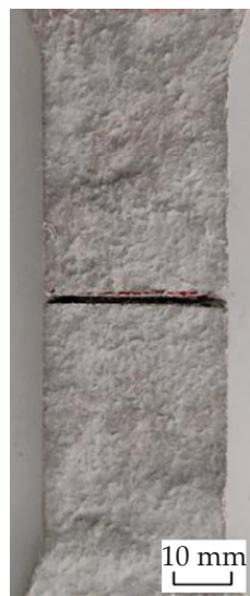
Figure 15. Failure mode of the single-seam tensile specimen.
