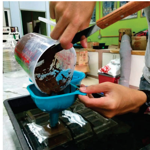
Figure 1. AAFA paste poured into mould in seawater.
