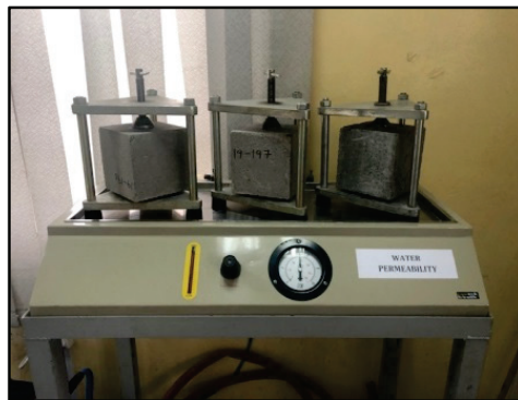
Figure 6. Water permeability test device.
