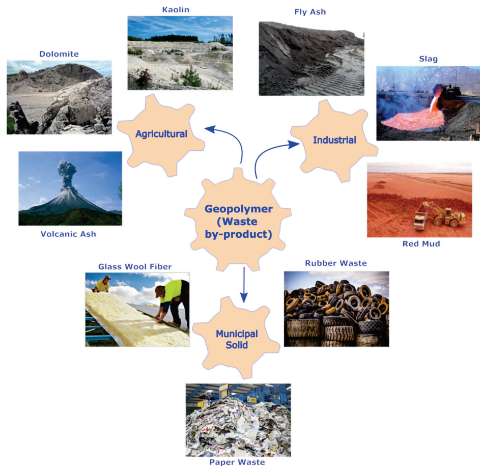
Figure 1. Common type of precursor materials used in geopolymer material.
