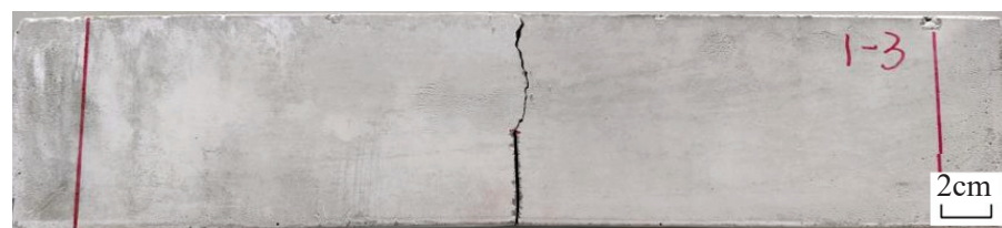
Figure 13. Failure mode of the three-point bending test specimen.
