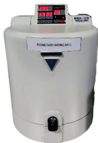
Figure 3. Planetary Mono Mill Pulverisette 6 can be used in the ball mill process.
