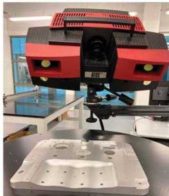
**Figure 5.** Automatic measurement data acquisition process set-up.
