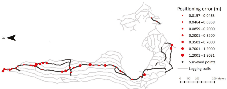
Figure 4. Distribution of absolute errors of positions recorded for u-blox ZED-F9P in control points.
