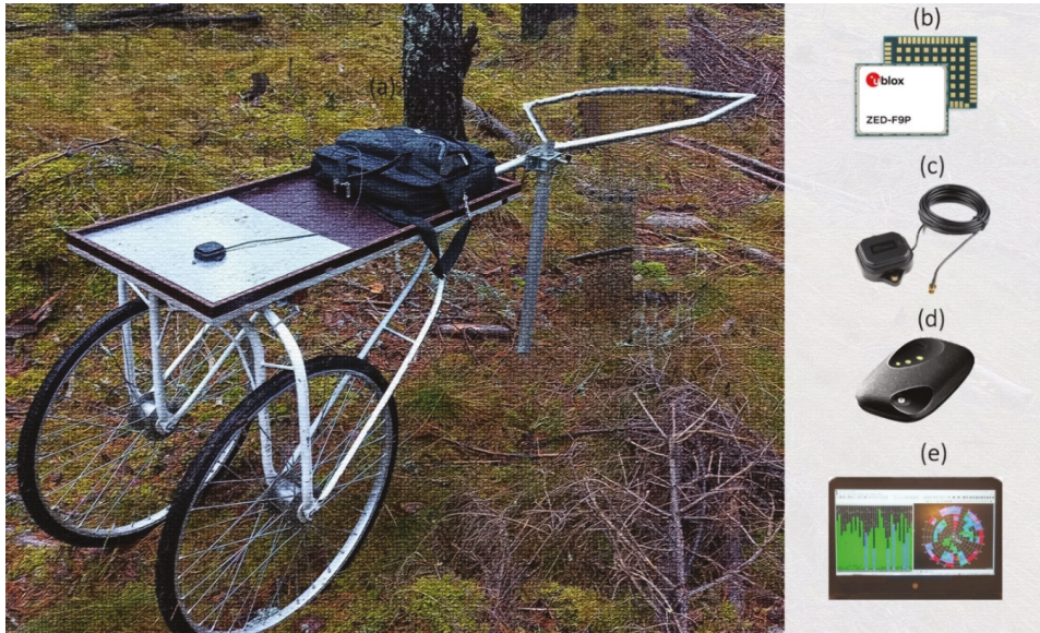
Figure 2. Compartments for field experiment: (a) research sully, (b) u-blox ZED-F9P, (c) Multi band GNSS antenna ANN-MB-00 (SMA), (d) modem, and (e) computer system.
