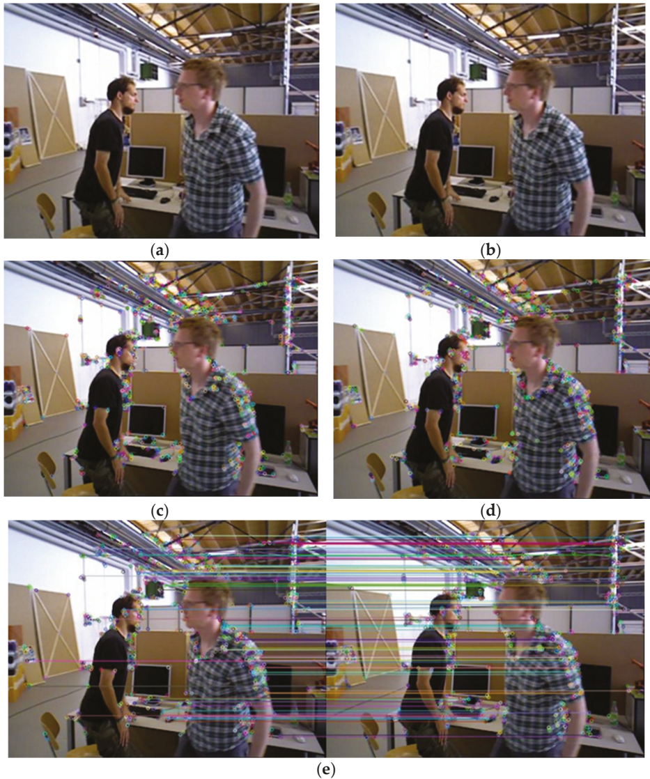
Figure 9. Results of feature extraction and matching based on ORB-SLAM2: (a) Original Figure 1; (b) Original Figure 2; (c) Feature points extracted before screening of original Figure 1; (d) Feature points extracted before screening of original Figure 2; (e) The ORB matching results of original Figures 1 and 2.
