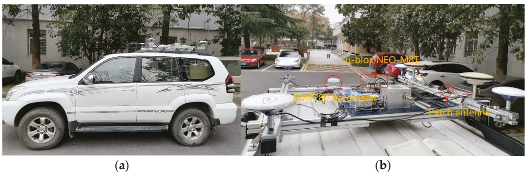
Figure 11. The mobile station hardware equipment site for kinematic vehicle experiment, including four geodetic GNSS receivers and antennas, NovAtel SPAN-FS GNSS/INS system, low-cost NEO-M8T receiver with a patch antenna, and a BMP280 barometer: (a) the experimental vehicle; (b) equipment setup diagram.
