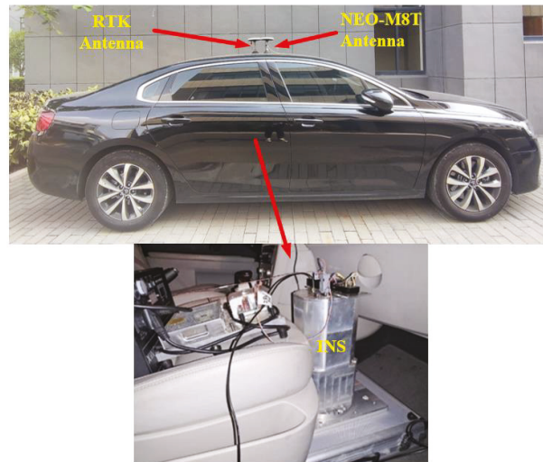
Figure 5. Data acquisition vehicle platform.
