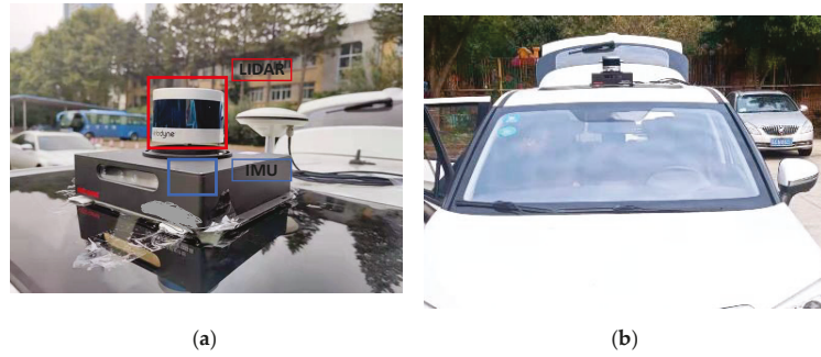
Figure 15. Our sensor suite. All have hardware time synchronization (a) IMU is in the LIDAR below. Integrated navigation device is used to gain ground truth. (b) The device is mounted on top of the vehicle.
