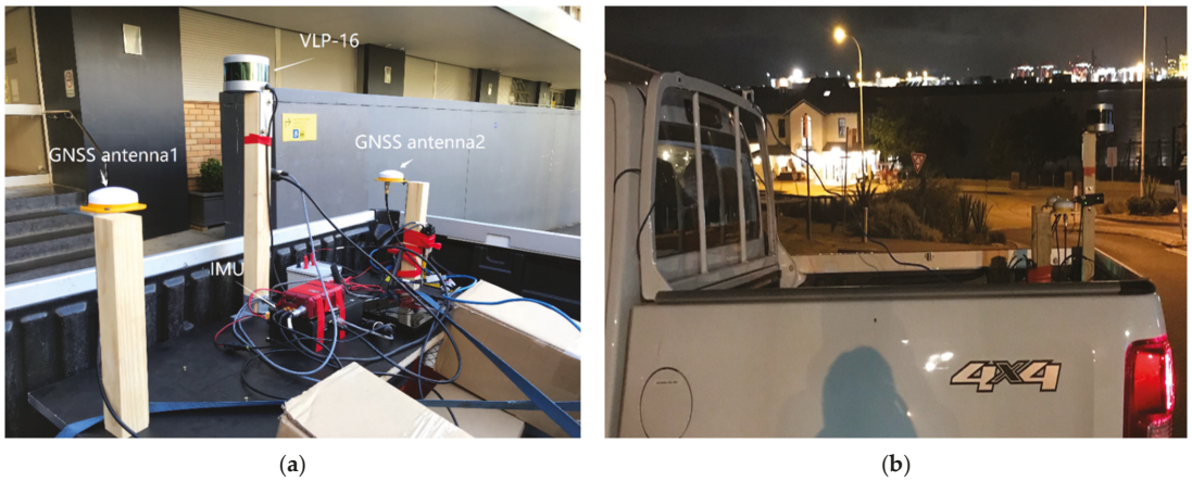
Figure 5. Experimental platform: (a) The multi-sensor system, (b) side view of the system installed within a vehicle.
