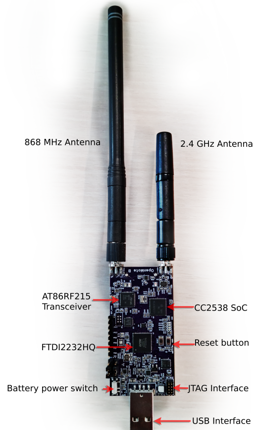
Figure 4. The OpenMote B used in parts of the experiment.
