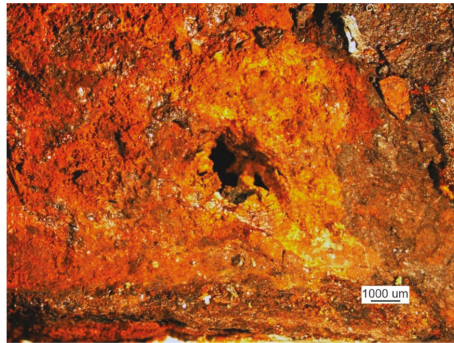
Figure 37. The deep corrosive pit is the presumed origin of the crack (handy-size bulk carrier 30185 DWT). Stereoscopic optical microscopy.
