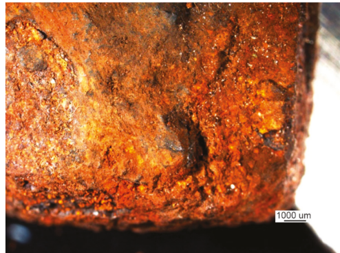
Figure 40. Corrosion pits at the edge of part 1 (handy-size bulk carrier 30185 DWT). Stereoscopic optical microscopy.
