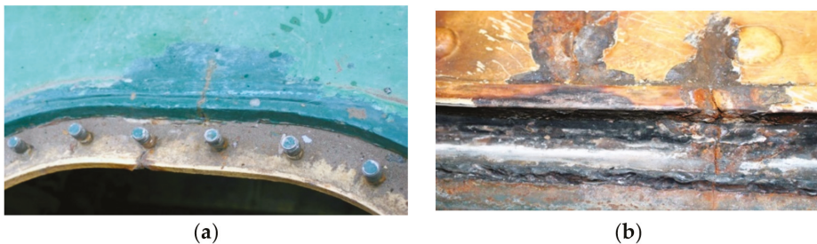
Figure 4. Pictures of origins of cracks: (a) view from the outside and (b) view from the inside of the tank (handy-size bulk carrier 30182 DWT). Macroscopic examination.
