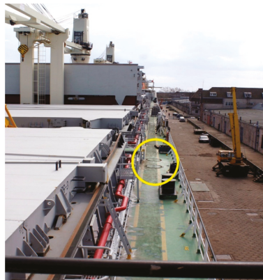
Figure 2. The main deck and tank inspection manhole covers for ballast tanks.
