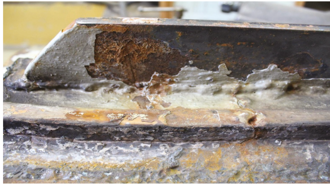
Figure 14. The crack in element IV (handy-size bulk carrier 30206 DWT). Macroscopic examination.
