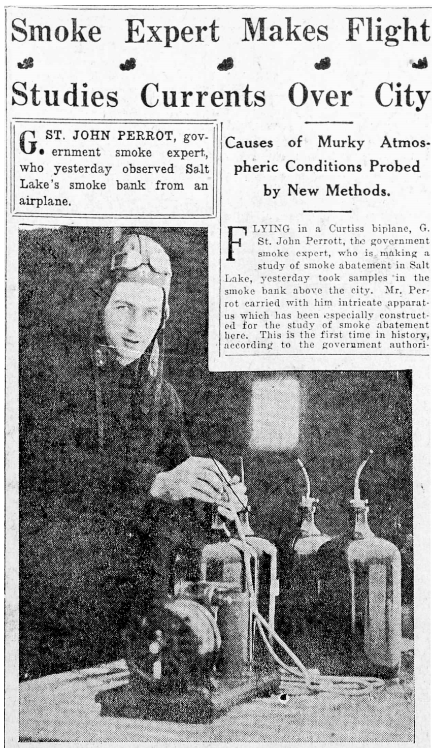
Figure 4. Photo of G. St. John Perrot and the sampling flasks used in the first aircraft sampling campaign to study SLC's air pollution, Salt Lake Tribune, 10 November 1919, digitalnewspapers.org [50].
