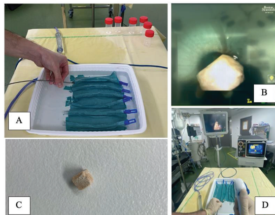
Figure 1. Experimental set up showing (A) Six polymer tubes, 17 cm length, closed on one side, 7 mm diameter, with an opaque tape on a tray with saline, used as a ureteral model (B) Endovision of the ureteral model with a Lithovue (Boston Scientific ® , Maple Grove, MN, USA) and a BegoStone on it (C) BegoStone 5 \times 5 \times 5 \text{ mm}^3 , dry weigh before and after the tests (D) Room display, using a Lithovue (Boston Scientific ® , Maple Grove, MN, USA). Irrigation was ensured by a combination of a gravity irrigation at 40 \text{cmH}_2\text{O} above the saline tray and a hand-assisted irrigation system.
